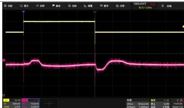
图9. LHR4025 CL=1uF Line Tran
