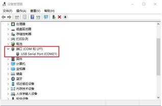
③. Set the serial port debugging parameters (Baud rate: 115200bps, data bit: 8bit, parity bit: no parity, stop bit: 1bit). (See the figure below)
