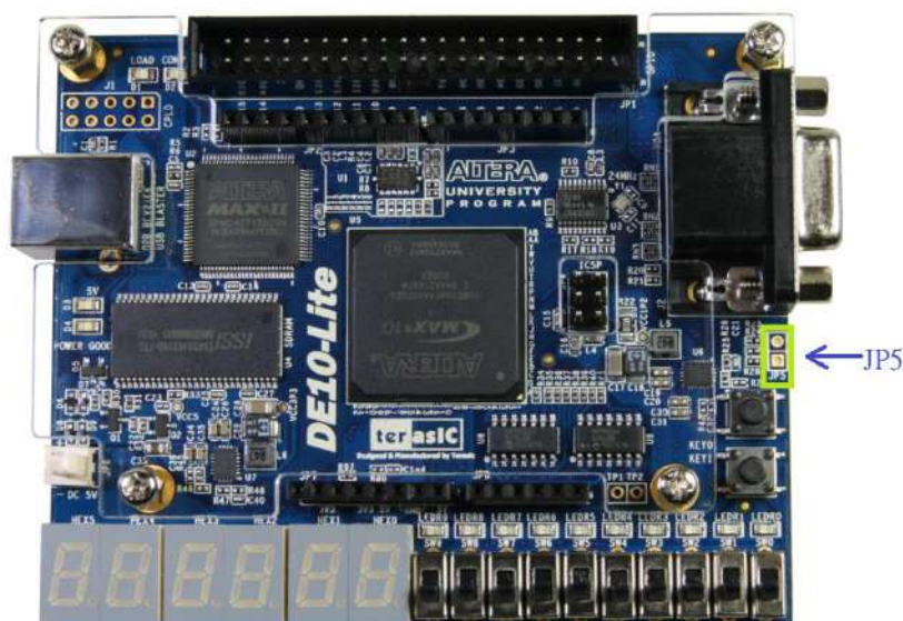
Figure 6-1 JP5 position on the DE10-Lite board.
