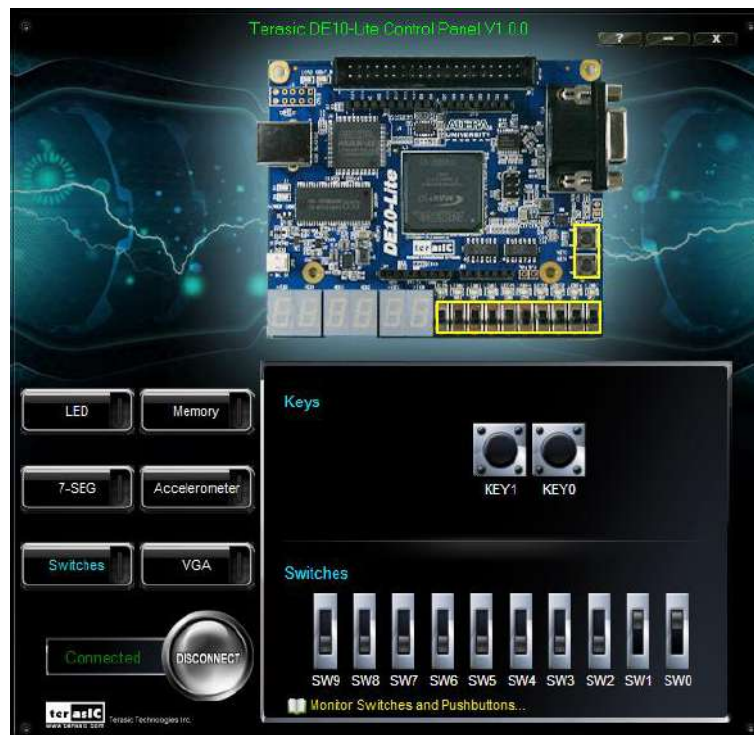
Figure 2-5 Monitoring switches and buttons
