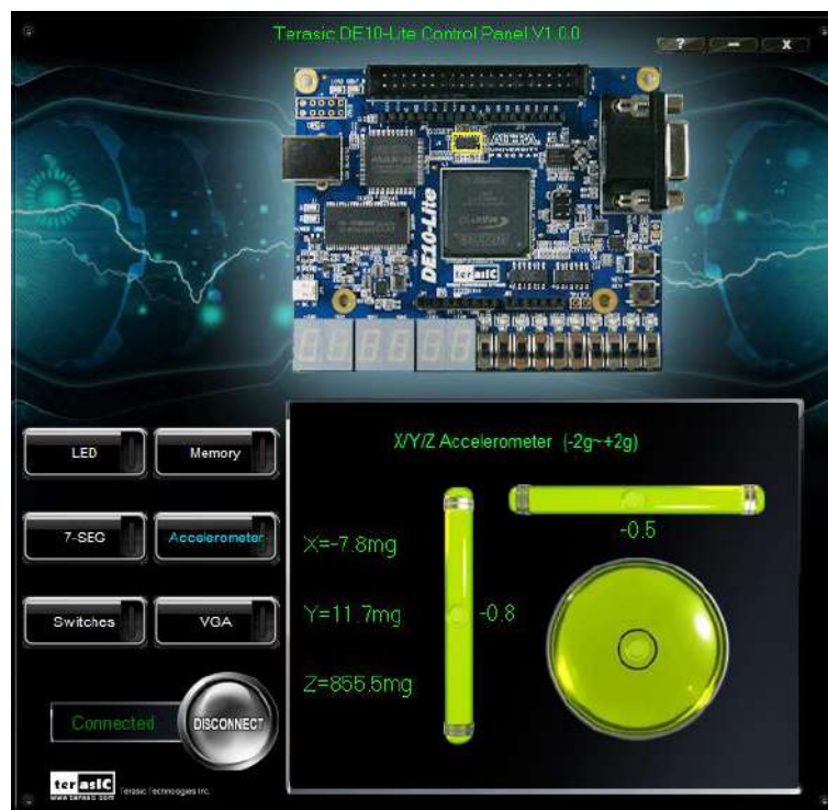
Figure 2-7 Level by G-Sensor
