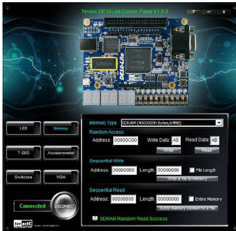
Figure 2-6 Accessing the SDRAM
