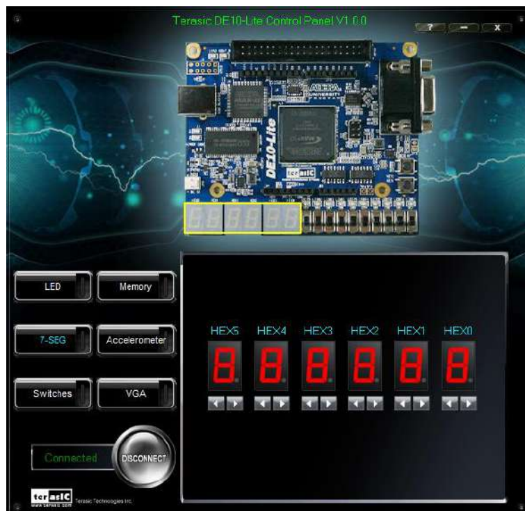
Figure 2-4 Controlling 7-SEG display
