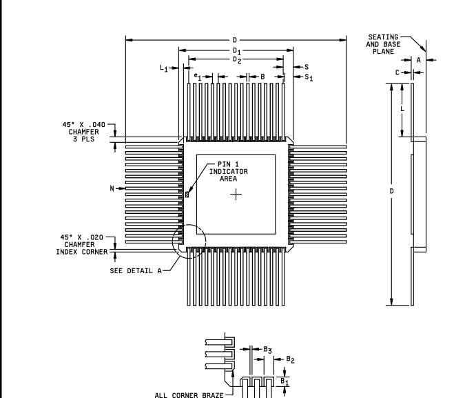
ALL CORNER BRAZE — PADS ARE 45° CHAMFER DETAIL A
