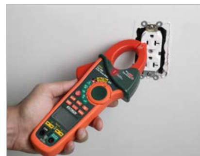
Non-Contact Voltage (NCV) Detection.
