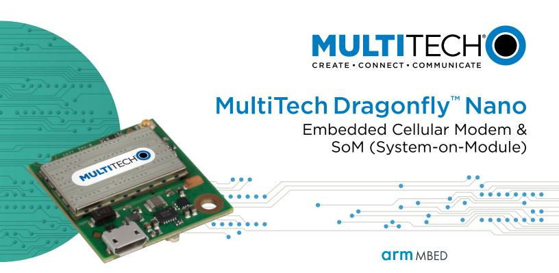
MultiTech Dragonfly™ Nano embedded cellular modems and SoMs are one of the industry's smallest form factor, end device approved, devices that can support a complete IoT operating system. The Dragonfly Nano is over 50% smaller, maintains plug compatibility and uses the same 40-pin board to board connector or USB connector found in the standard sized Dragonfly family; providing a full range of connectivity and carrier options.
