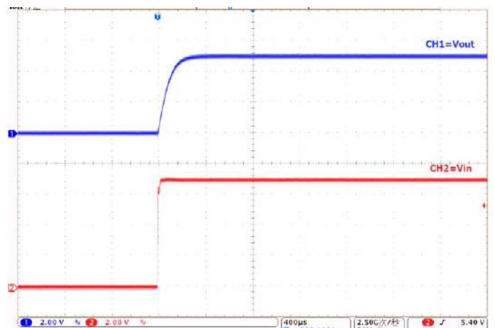
Power-Up at V_{OUT}=5.0V : (I_{OUT}=150mA)
