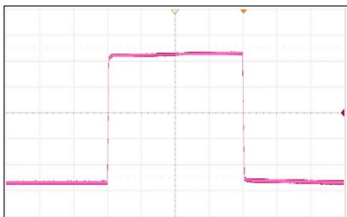
Figure 18. Large-Signal Pulse Response
