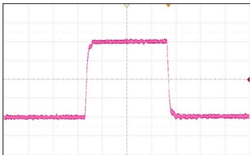
Figure 24. Small -Signal Pulse Response
