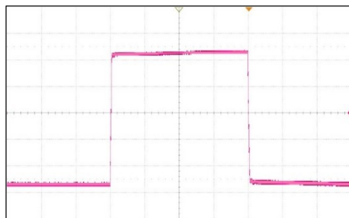
Figure 19. Large-Signal Pulse Response
