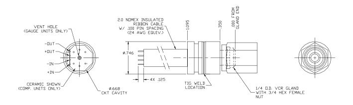
Note1: Non-concentricity effects at the diaphragm weld area may cause run out of up to ±0.006" between the upper and lower portions of the sensor body. (It is recommended to use a counter bore in the mating bore used with this device to allow for this non-concentricity.)
